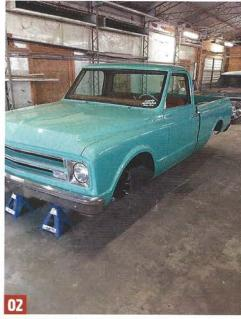
O2 Jack up the truck and support it with jack stands. Make sure the truck is level, which is critical to getting the molding affixed properly. Remove all four wheels and front inner fender wells so that you can access the fender and bedside molding studs.
