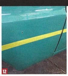
12 Using a 1/8-inch bit, drill a pilot hole in the three marked locations. Then drill the final mounting hole using a 3/8-inch bit. We prefer to use a step bit, but a standard drill bit will also work. You can now final-install the molding using the provided hardware. Be sure all of the molding lines up with the reference tape before tightening.
