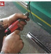
14 Measure 1 1/4 inches down from the factory body lines and mark the final clip holes. Drill a 1/8-inch pilot hole in each of the final marked locations, and follow with a 3/8-inch bit. Install the molding, lining it up with the reference line. Repeat this for the rear cab corner pieces.
