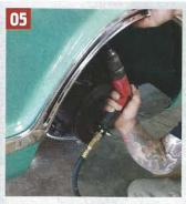
**05** After the molding is properly aligned and securely taped to the wheel opening, drill a 1/8-inch hole in each of the five positions on the inner wheel lip opening. Start in the center and move outward.
