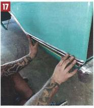
16-17 Now that the wheel opening molding is in place, insert the clips into the front and rear bedside molding. Make sure to place the three provided clips evenly along each piece. Follow the same steps for the remaining wheel areas, making sure to measure 1½ inches down from the body line, aligning the molding with the tape line.
